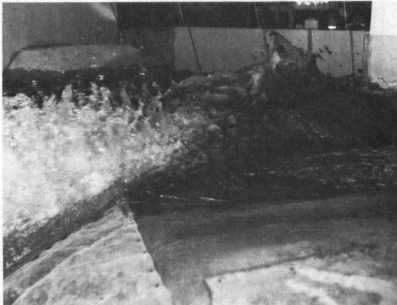
b. Exit channel at Q = 510 \text{ m}^3/\text{s} (18 000 \text{ft}^3/\text{s} ). Tailwater is washed out and velocity is very high at the model tailgate. Photo P801-D-79464
