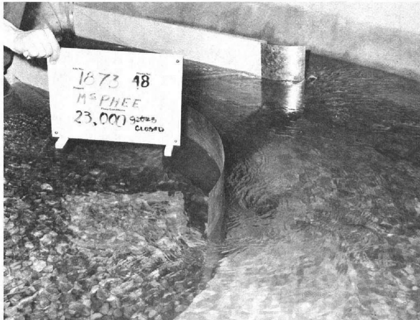
b. Curved guide walls added, Q = 650 \text{ m}^3/\text{s} ( 23\,000 \text{ ft}^3/\text{s} ). Photo P801-D-79451
