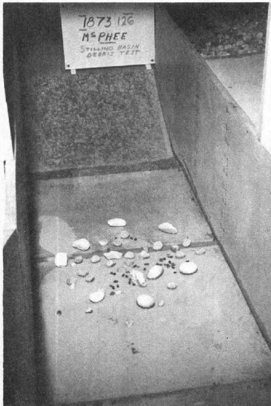
c. Location of debris after 45 minutes model operation at Q = 200 \text{ m}^3/\text{s} ( 7000 \text{ ft}^3/\text{s} ). Note 75-mm rocks washed out and deposited downstream from the center of the flip lip. Photo P801-D-79479
