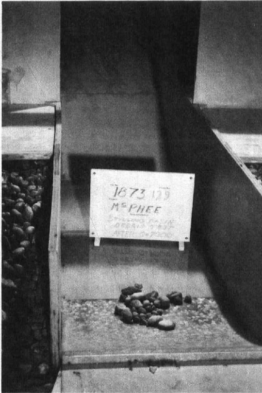
a. Debris placed in basin before stilling basin debris tests. Downstream view. Photo P801-D-79477
