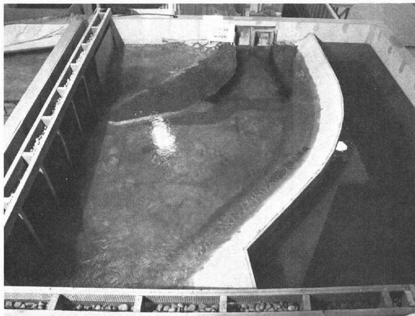
b. Q = 940 \text{ m}^3/\text{s} (33 130 \text{ft}^3/\text{s} ), inflow design flood, reservoir elevation = 2111.23 m (6926.6 ft). Photo P801-D-79457
