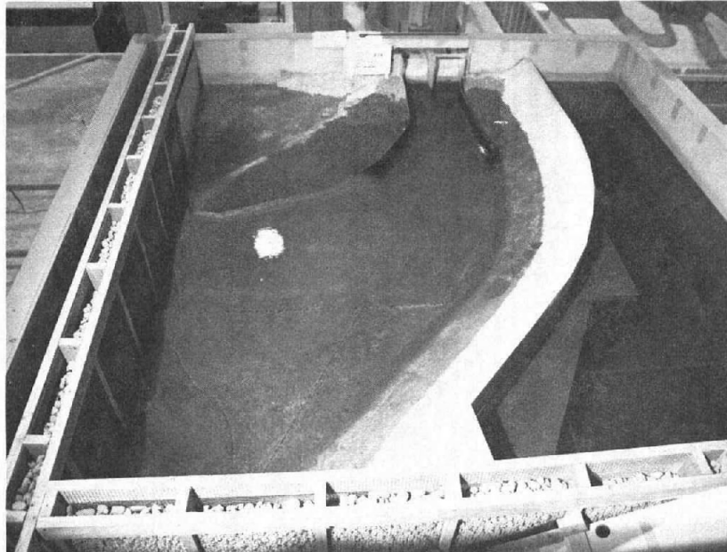
a. Q = 375 \text{ m}^3/\text{s} (13 300 \text{ft}^3/\text{s} ), 100-year flood, reservoir elevation = 2110.97 m (6925.75 ft), gate opening = 2.62 m (8.6 ft). Photo P801-D-79456
