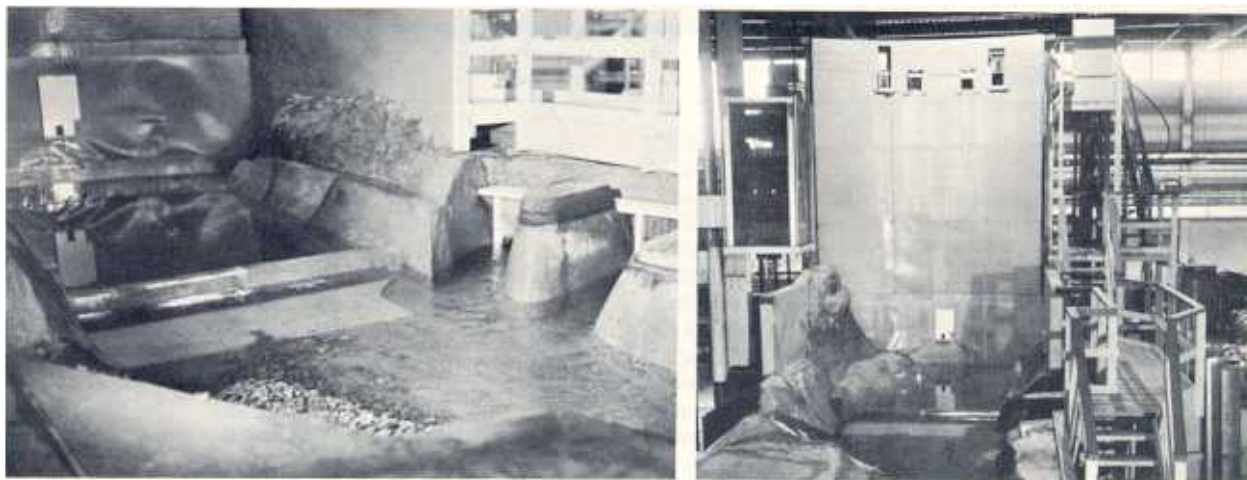
FIGURE 44.—Operation of the recommended design with powerplant discharge only ( Q=5,200 cubic feet per second).
