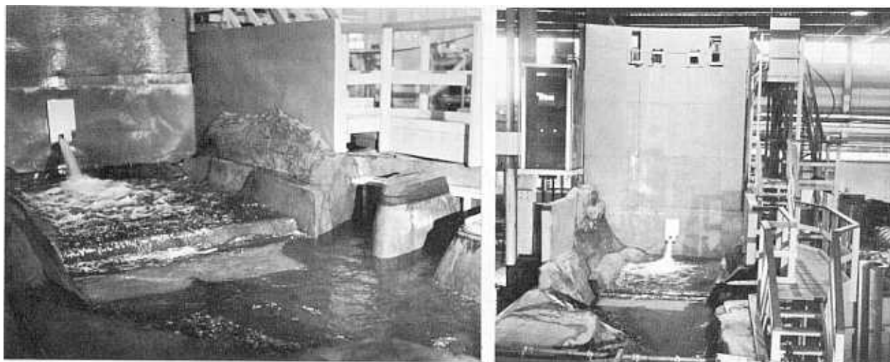
FIGURE 45.—Operation of the recommended design with discharges from the outlet works and the powerplant (outlet works Q=1,500 cubic feet per second and powerplant Q=5,200 cubic feet per second).
