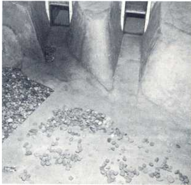
FIGURE 37.—View of area below the weir after 1 hour at spillway Q=34,400 cubic feet per second. (Maximum design discharge for the spillway.)
