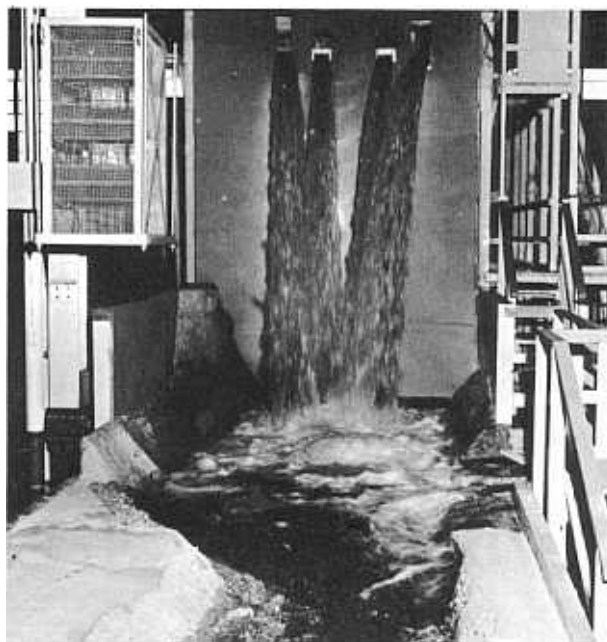
FIGURE 29.—View showing flow characteristics in the stilling basin following removal of the piers from the weir structure and extension of the stilling basin lining. Maximum design discharge.
