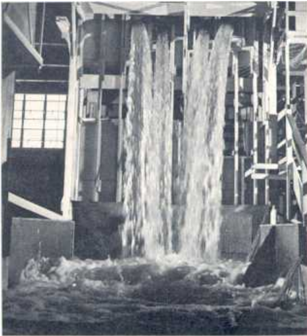
FIGURE 16.—Test on spillway of alternate design with inside conduits tipped 27° downward. Reservoir elevation 7165 with gates fully open (approximate Q=40,000 cubic feet per second).
