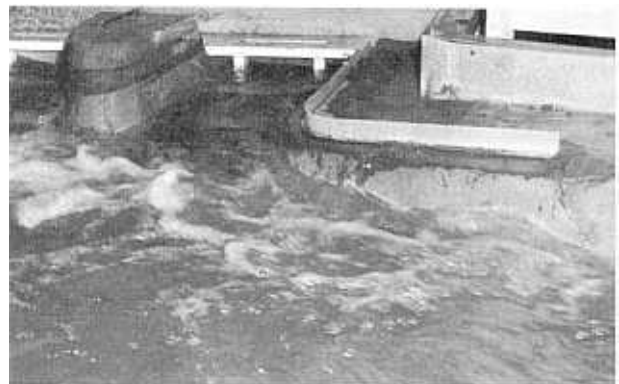
FIGURE 23.—Test of floodwall protection around visitors' center (approximate discharges: spillway Q=26,000 cubic feet per second, outlet works Q=1,500 cubic feet per second, and powerplant Q=5,200 cubic feet per second).
