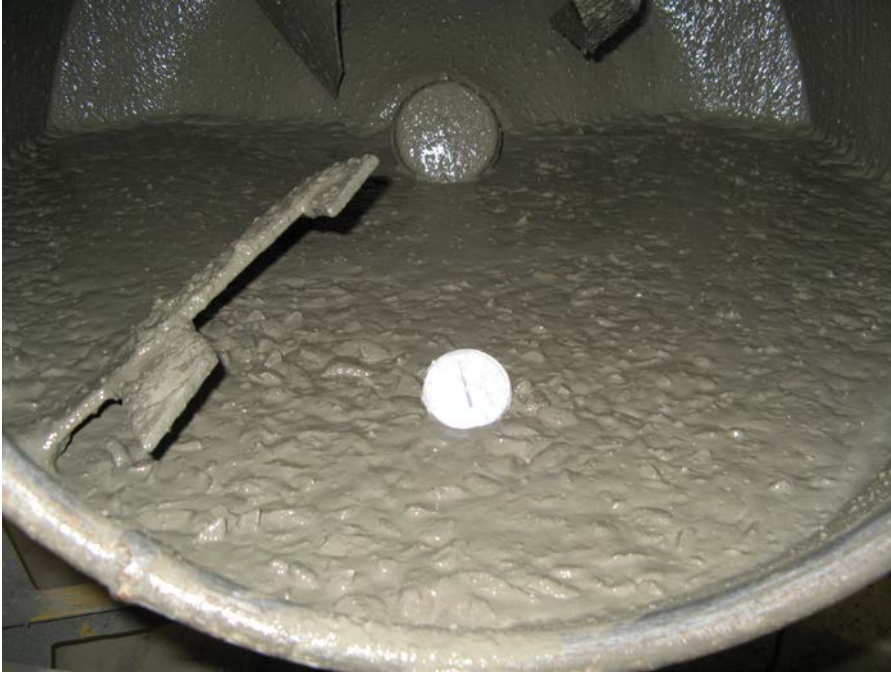
Appendix D Figure 1 - Concrete in the laboratory mixer made with materials from the Deer Creek Dam Spillway Modification project.
