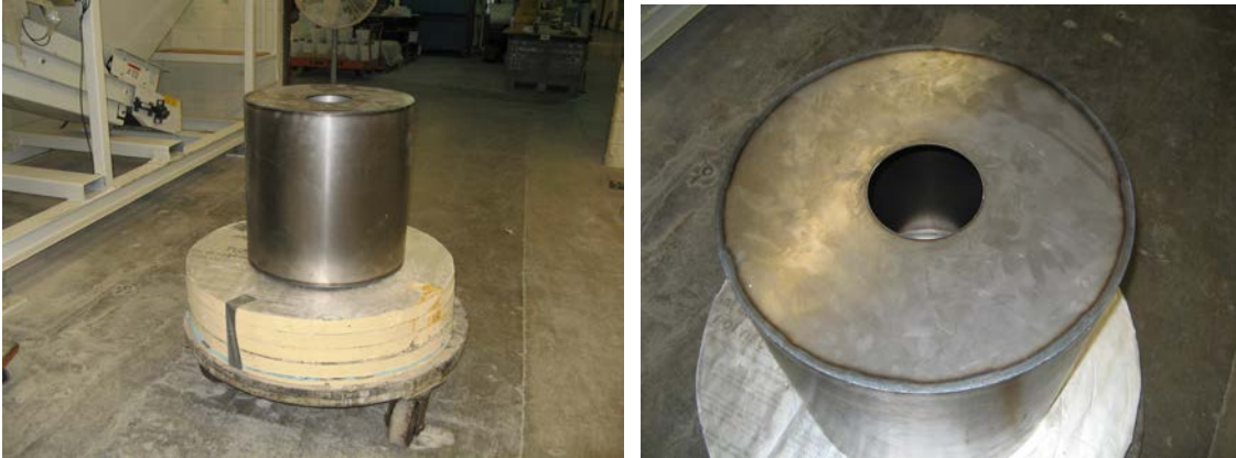
Appendix D Figure 3 - Standard USBR 4911 temperature rise container (surrounded with insulation after concrete is added).
