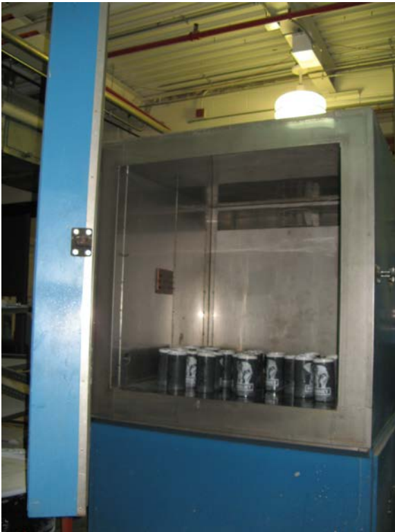
Appendix D Figure 6 - In-situ cure strength specimens cured inside a small environmental chamber programmed with the actual Deer Creek Dam Spillway temperature curve.
