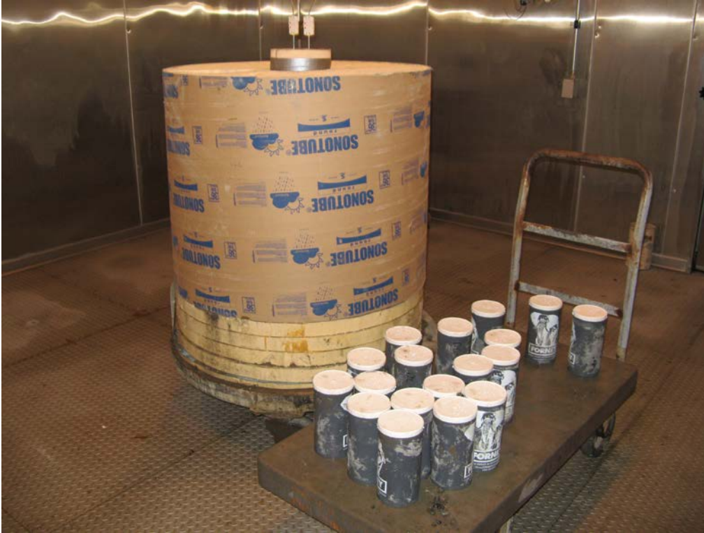
Appendix D Figure 5 - USBR 4911 Adiabatic Temperature Rise test in progress with companion adiabatic strength specimens (inside environmental chamber). The environmental chamber temperature is matched to the internal temperature inside the insulated temperature rise container.
