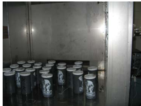
Appendix D Figure 6 - In-situ cure strength specimens cured inside a small environmental chamber programmed with the actual Deer Creek Dam Spillway temperature curve.
