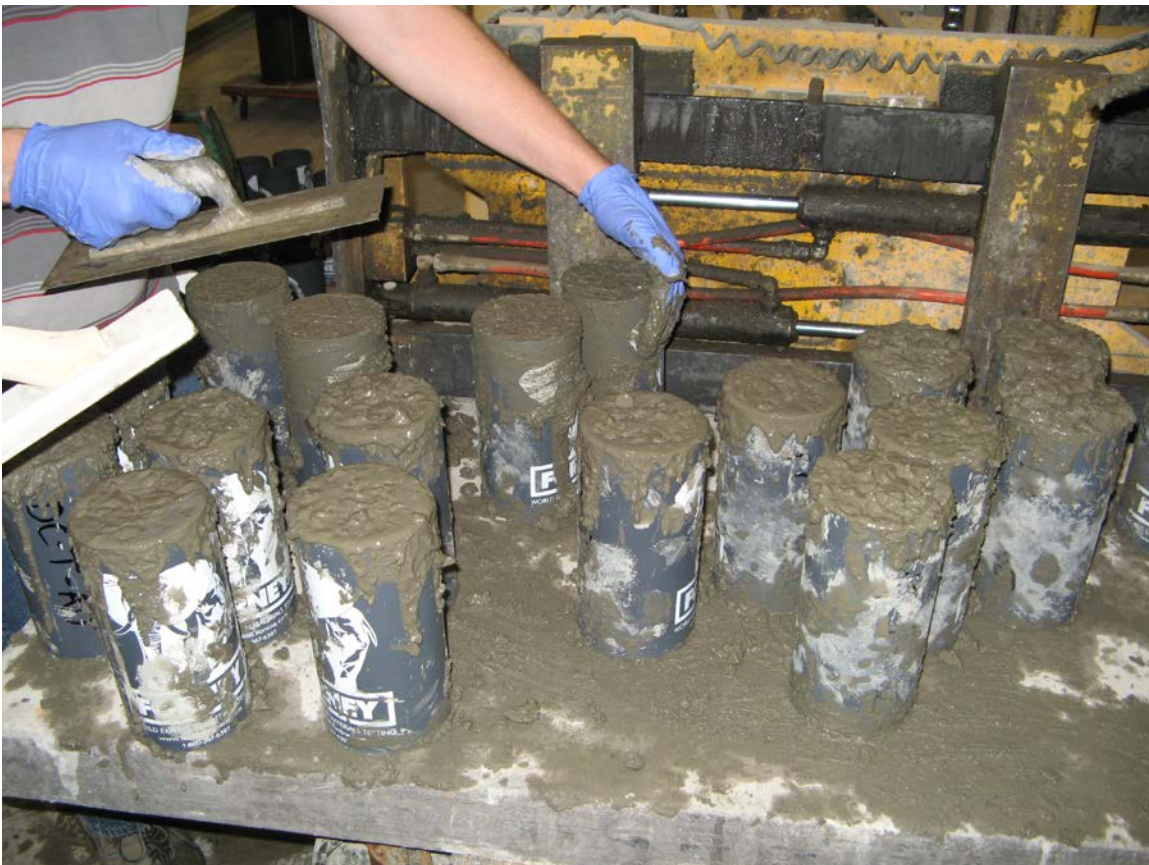
Appendix D Figure 4 - Making 4-by 8-inch concrete specimens for compressive strength and elastic properties testing.
