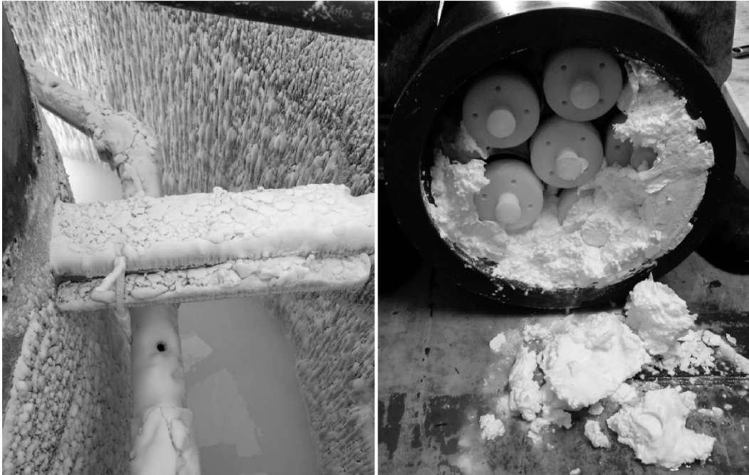
Figure 20. Calcium sulfate deposition in the precipitator and the candle filter.
