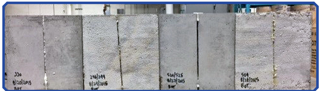
Injection of polyurethane grout in test tank.
