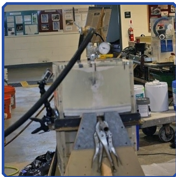
Test tank after AV-330 was used to seal crack.
