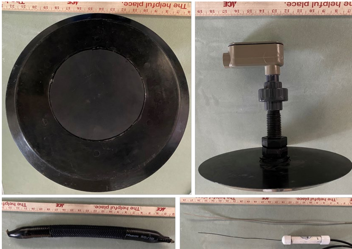
Photo 36. Typical ICCP anodes. MMO flush mounted disk anode (top), polymer sausage anode (bottom left), and MMO wire anode (bottom right)
