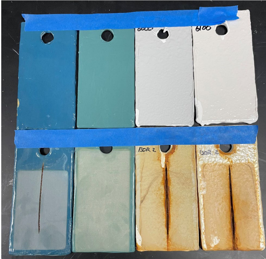
Photo 28. Test panels after 5040 hours of UV exposure
