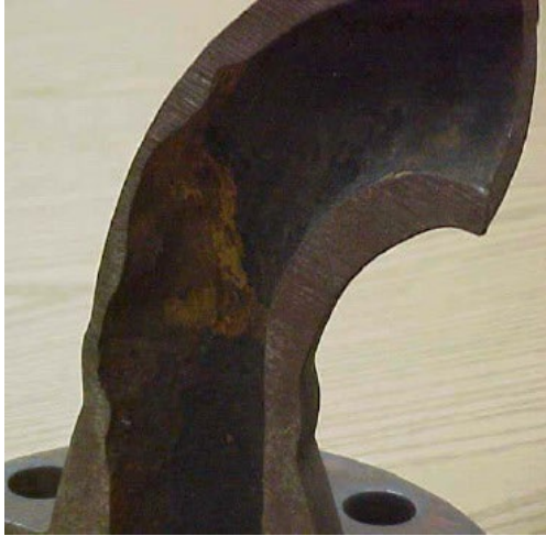
Photo 7. Pipe showing how high turbulence flow can cause erosion corrosion
