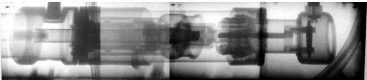
Figure 8-4. Radiographic image of a circuit breaker
