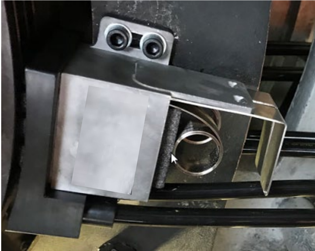
Photograph 3.—Collector ring spring fed stoning jig and integral vacuum assembly.
