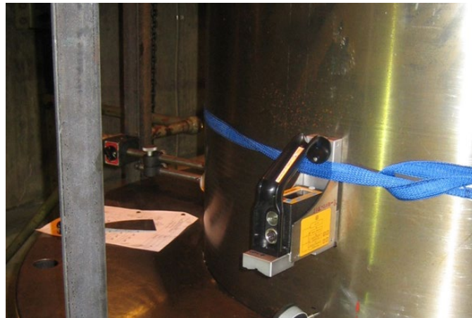
Figure 20.—Precision level attached to shaft with strap.
