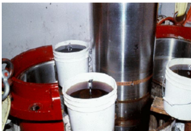
Figure 14.—Plumb wire setup.
