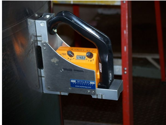
Figure 19.—Precision level with magnetic base.
