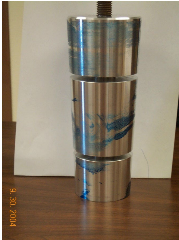
Photo 6.—Wicket gate shear pin.
