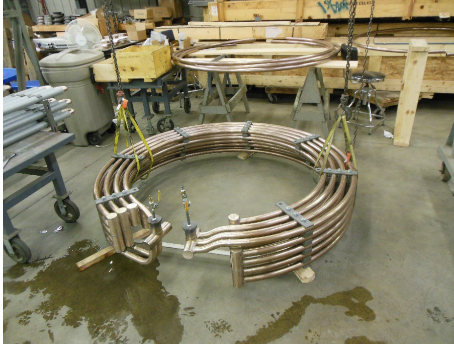
Photo 16.—Cooling coil for a guide bearing.
