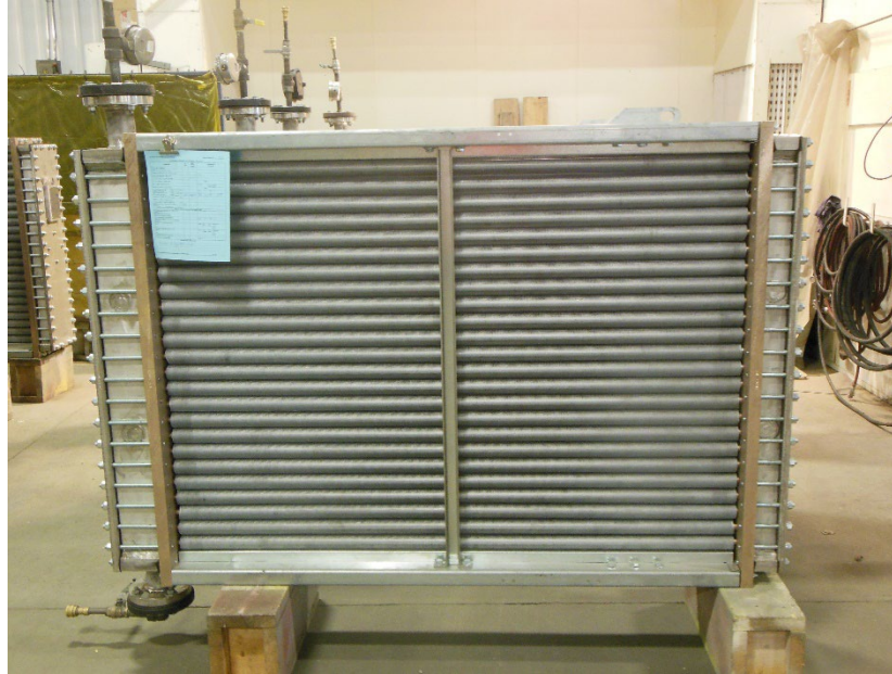
Photo 15.—Generator air cooler.
