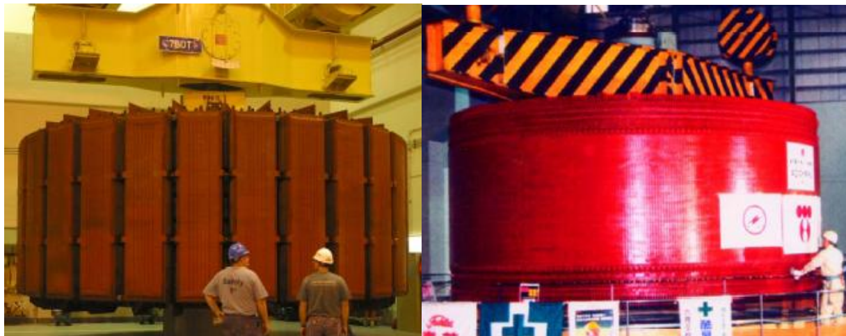
Figure 4-6. Single-Speed Rotor (Left) and Variable-Speed Rotor (Right)
