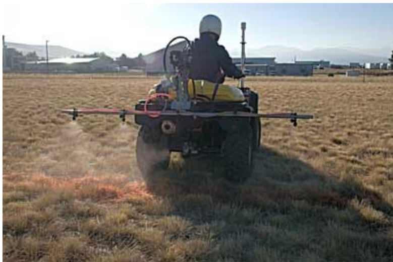
Figure 2-1. Example of boom sprayer nozzles producing uniform spray of a treated area (USDA 1999).
