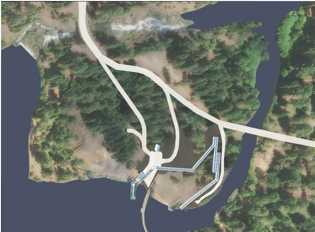
Figure 1. Close-up of the project area, where a new access road and the new fish ladder would be constructed on the north side of Clear Creek Dam
