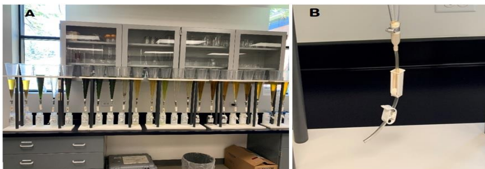
Figure 1: A. Cones are set up with samples. B. Close-up image of the closed roller clamp and the secondary clamp in place on the tubing.
