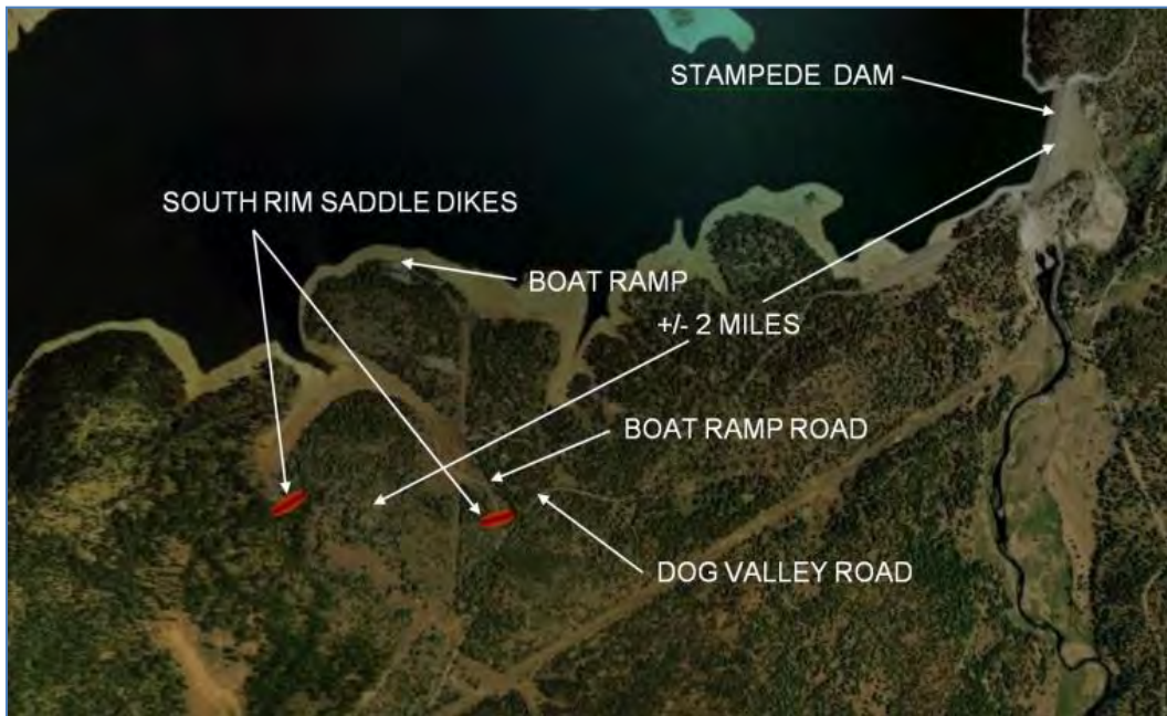
Figure 2-7.—Plan view of new saddle dikes for low areas on the south reservoir rim.
