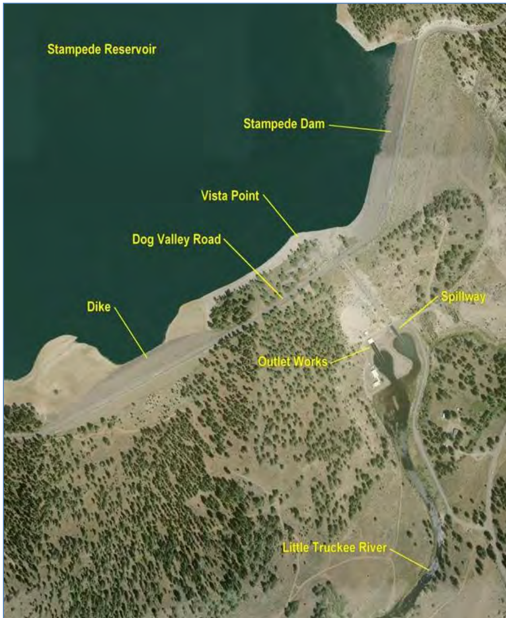
Figure 1-3.—Stampede Dam features.
