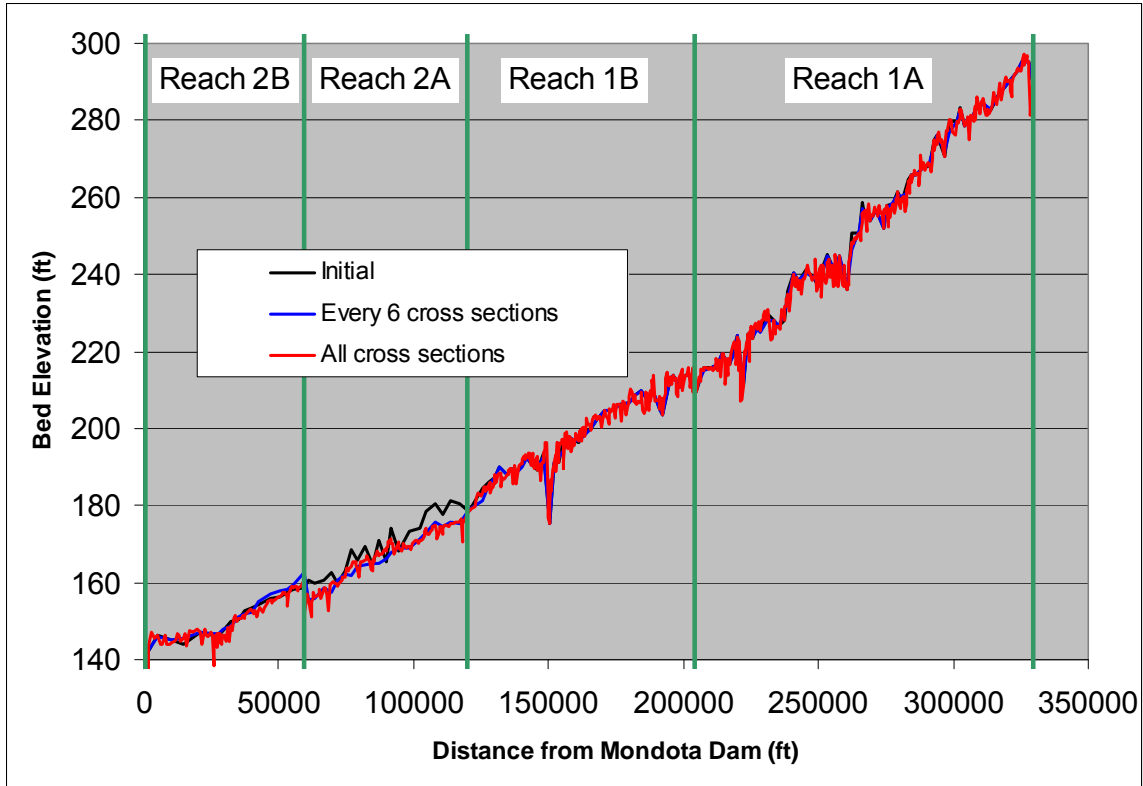
Figure C-9. Bed Profiles Simulated with Different Cross-Section Numbers
