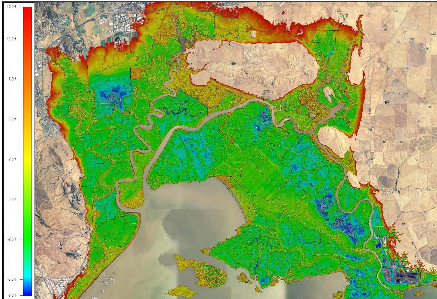
Figure 4-2 Suisun Marsh LiDAR data used in the model calibration – elevations shown in the color scale are in feet (NGVD29).
