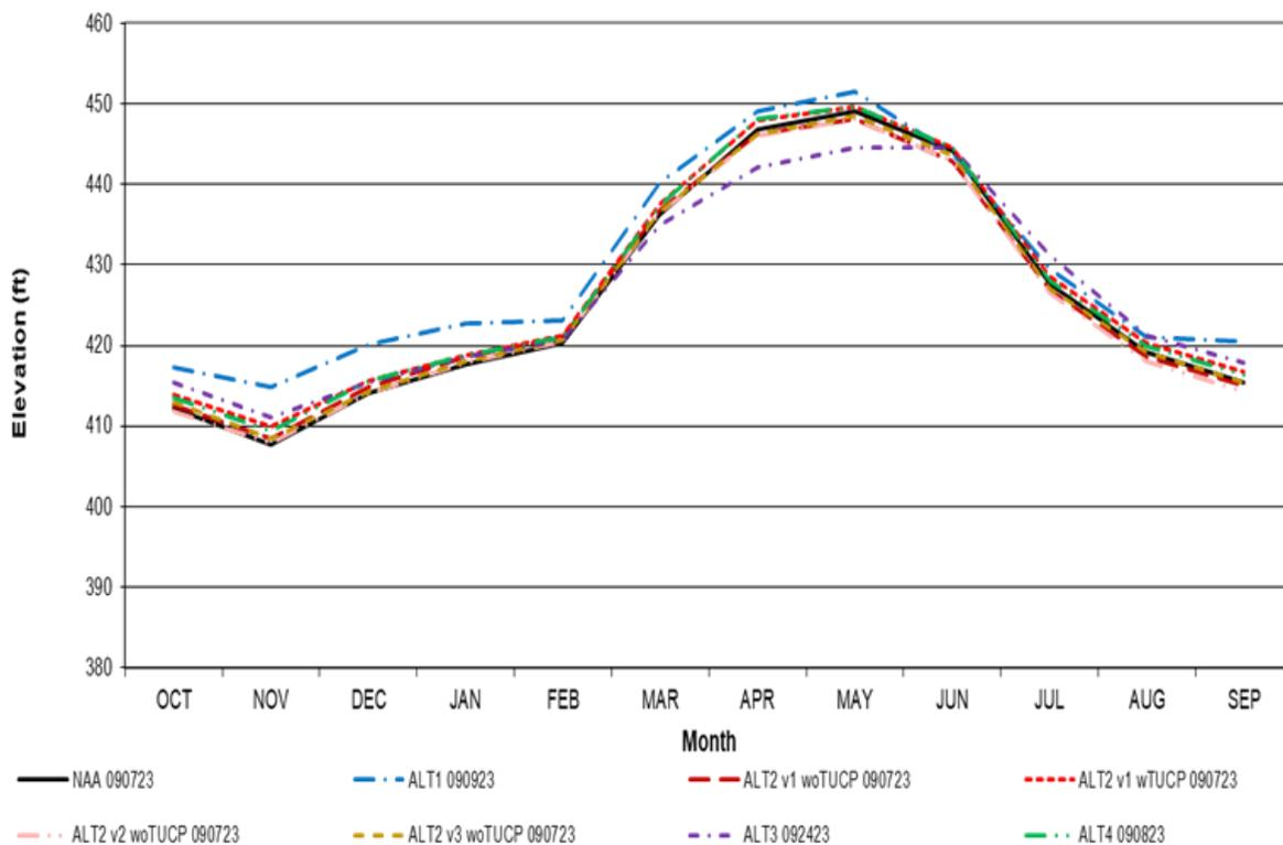
Figure S-7. Folsom Reservoir Long-Term Average Water Level Elevation
