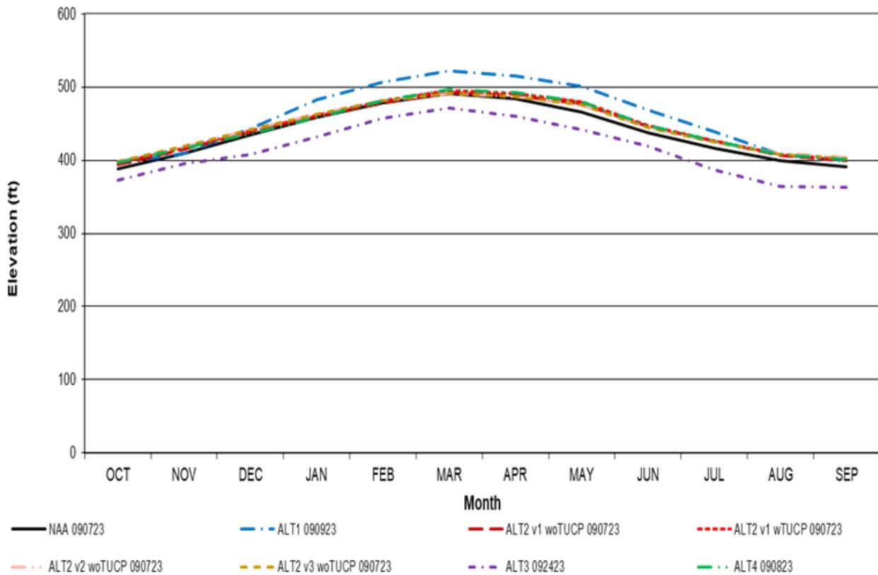
Figure S-14. San Luis Reservoir Long-Term Average Water Level Elevation
