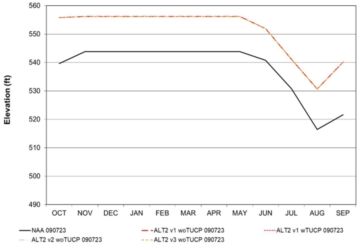
Figure S-31. San Luis Reservoir Alternative 2 Long-Term Average Maximum Water Level Elevation
