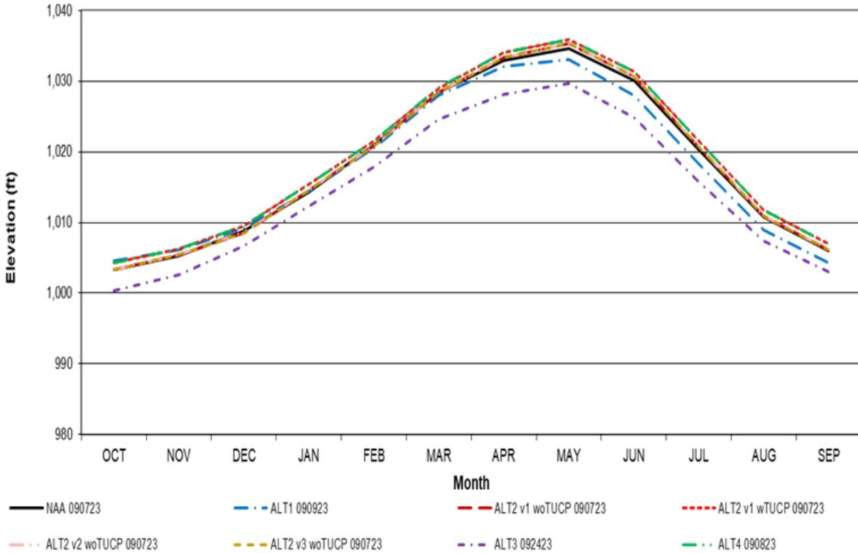
Figure S-10. New Melones Reservoir Long-Term Average Water Level Elevation
