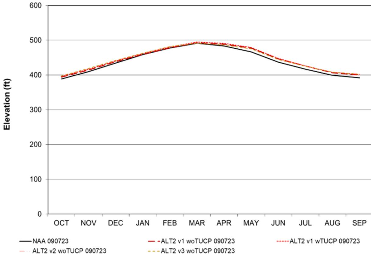
Figure S-29. San Luis Reservoir Alternative 2 Long-Term Average Water Level Elevation
