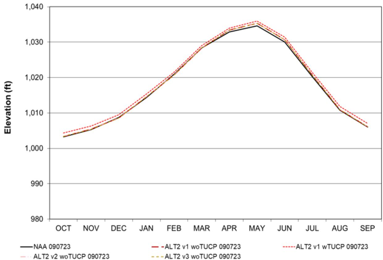
Figure S-25. New Melones Reservoir Alternative 2 Long-Term Average Water Level Elevation
