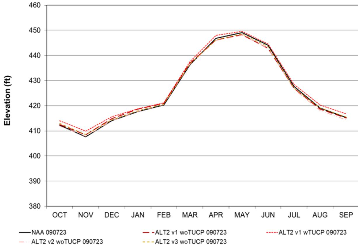
Figure S-21. Folsom Reservoir Alternative 2 Long-Term Average Water Level Elevation
