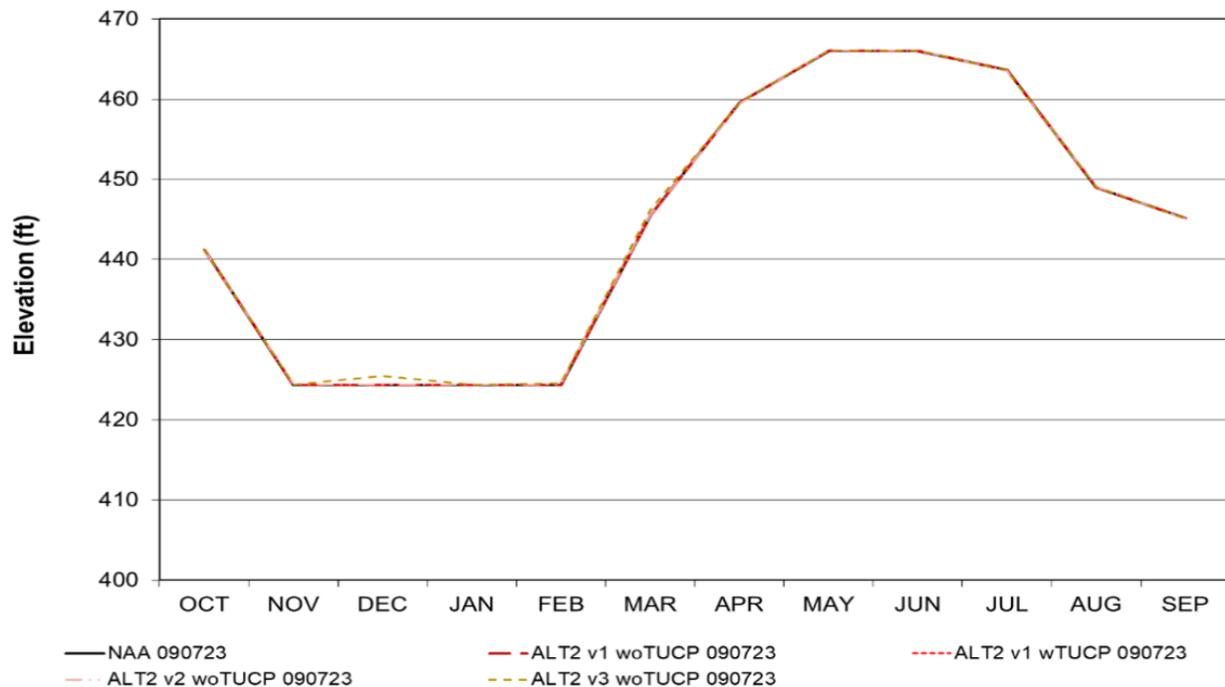
Figure S-23. Folsom Reservoir Alternative 2 Long-Term Average Maximum Water Level Elevation
