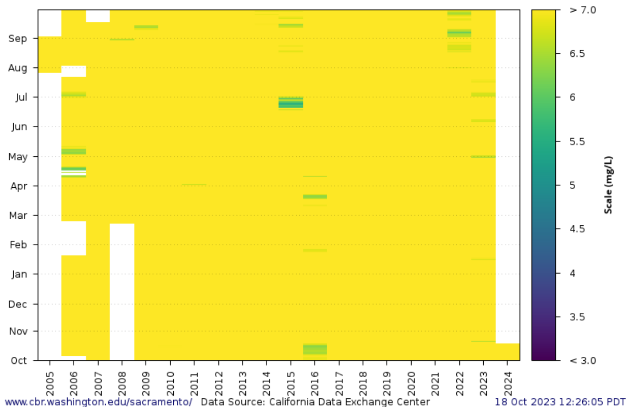
WY 2005-2024 SJR San Joaquin R, McCune Station nr Vernalis Daily Average Dissolved Oxygen (mg/L) Observed Range 5.54 : 15.96
