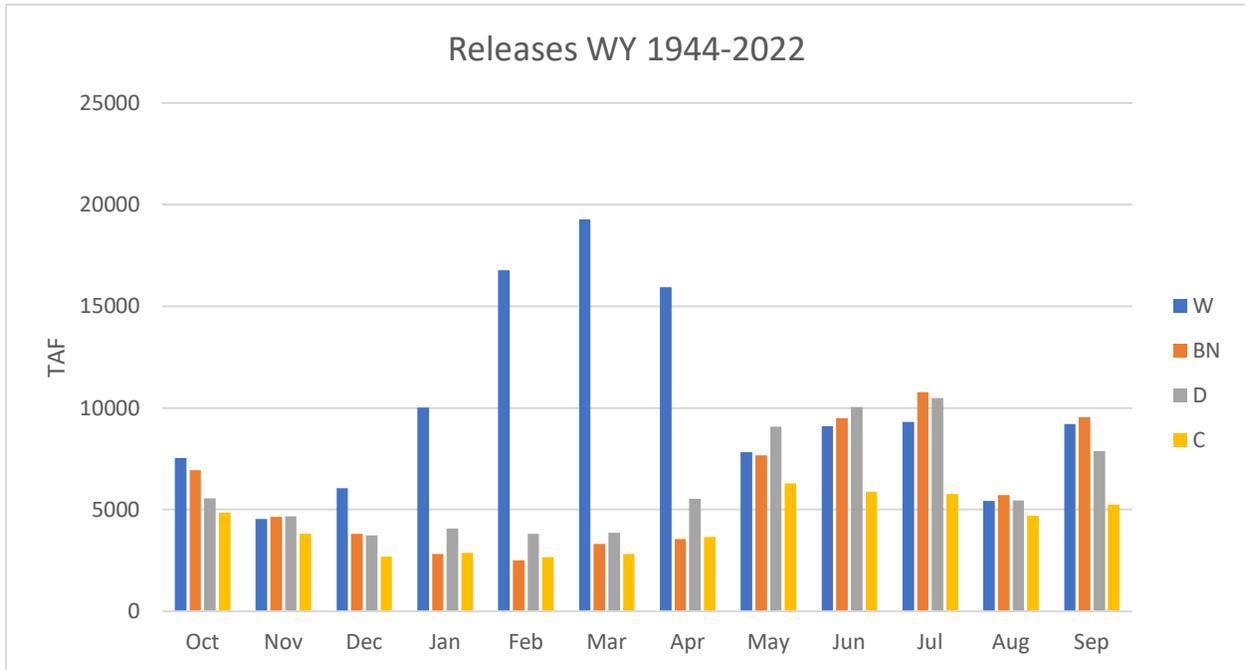
Figure L-1. Monthly releases from Shasta Dam by water year type for water years 1944 – 2022
