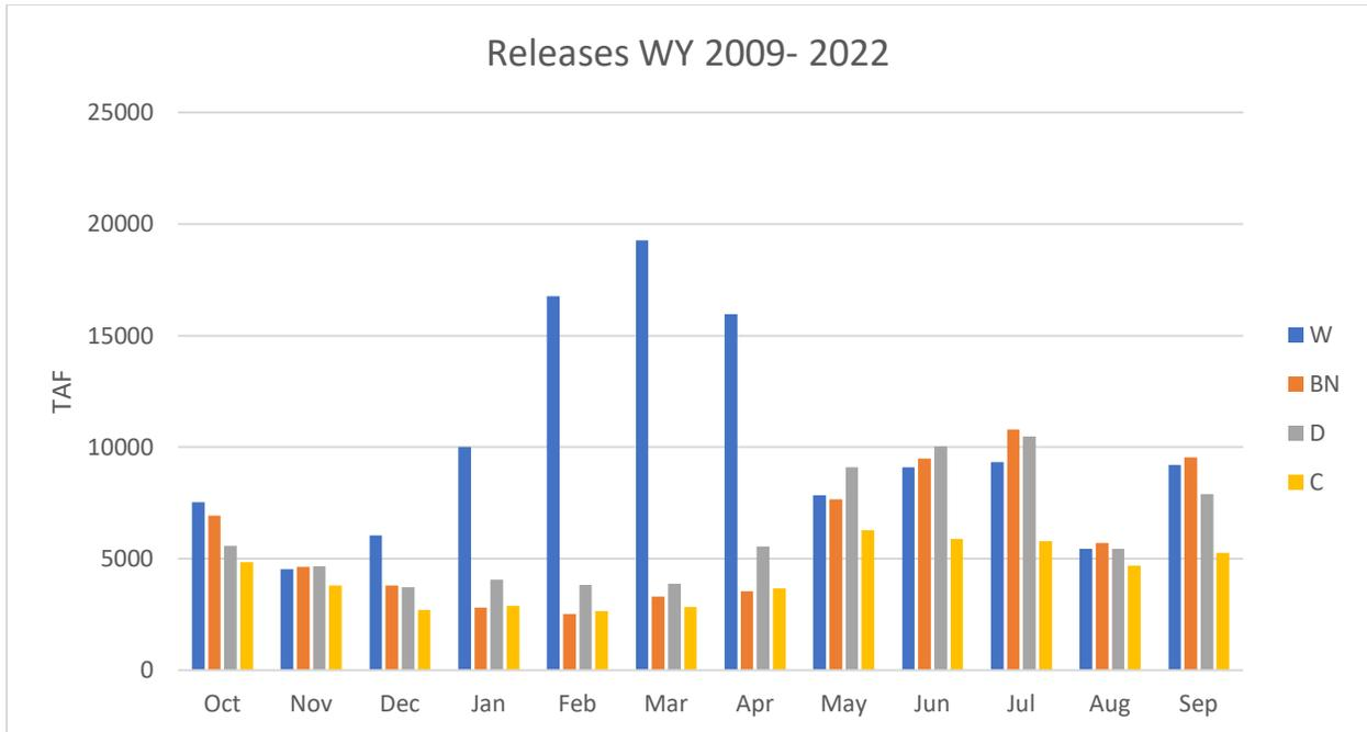
Figure L-2. Monthly releases from Shasta Dam by water year type for water years 2009 – 2022
