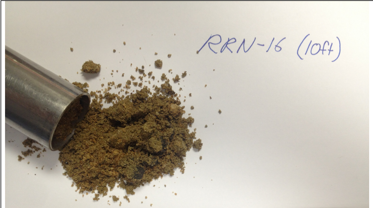
Photograph 7 Soil Sample RRN-16 from CPT, Depth of 10ft, Poorly Graded Sand
