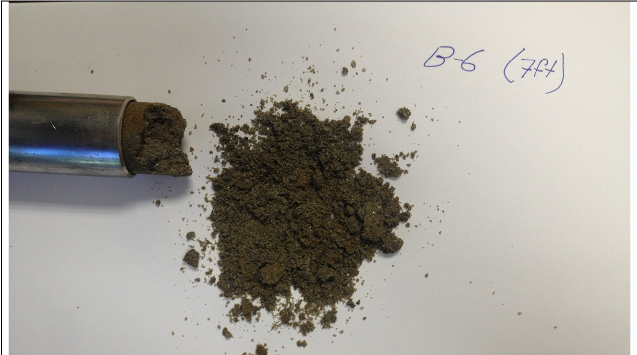
Photograph 1 Soil Sample B-6 from CPT, Depth of 7ft, Well Graded Sand with Silt
