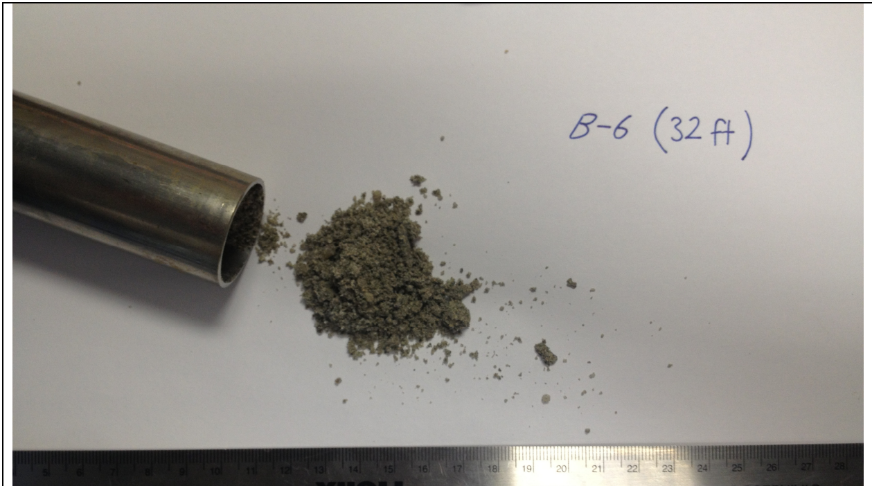
Photograph 3 Soil Sample B-6 from CPT, Depth of 32ft, Poorly Graded Sand
