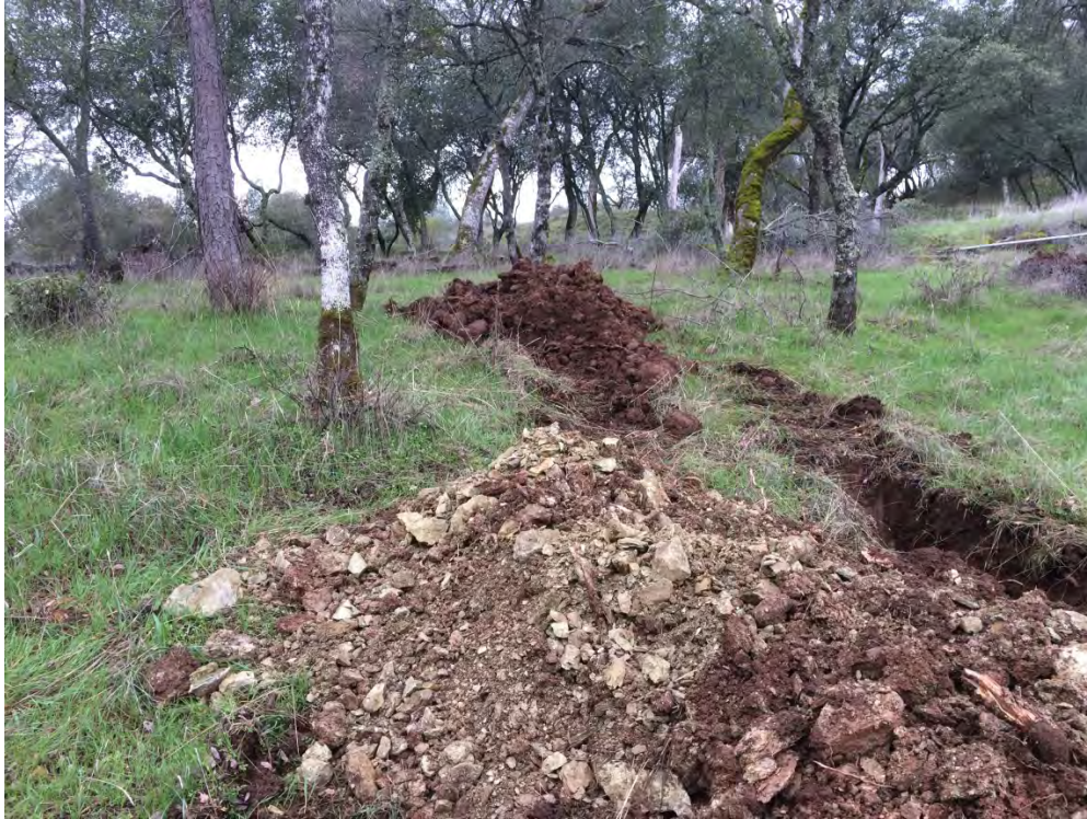
Photo 5 – Geologic contact between Mehrten formation and ultramafic rock, trenches T-12 and T-13.
