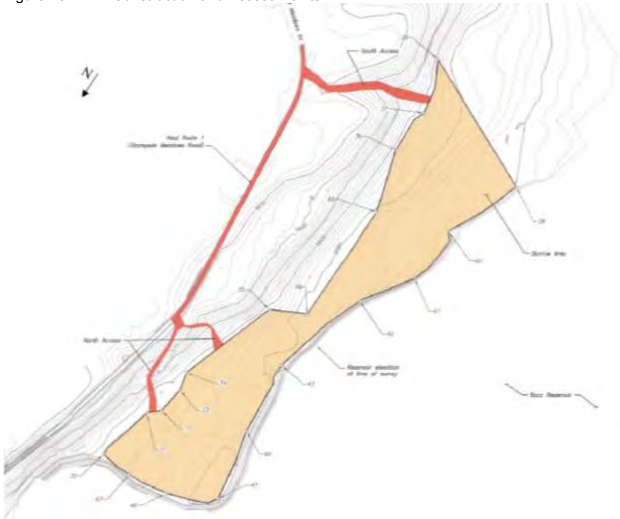
Figure 16. IRBA Construction and Access Points
