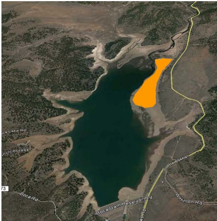
Figure 11. Proposed Action Alternative in-reservoir borrow area
