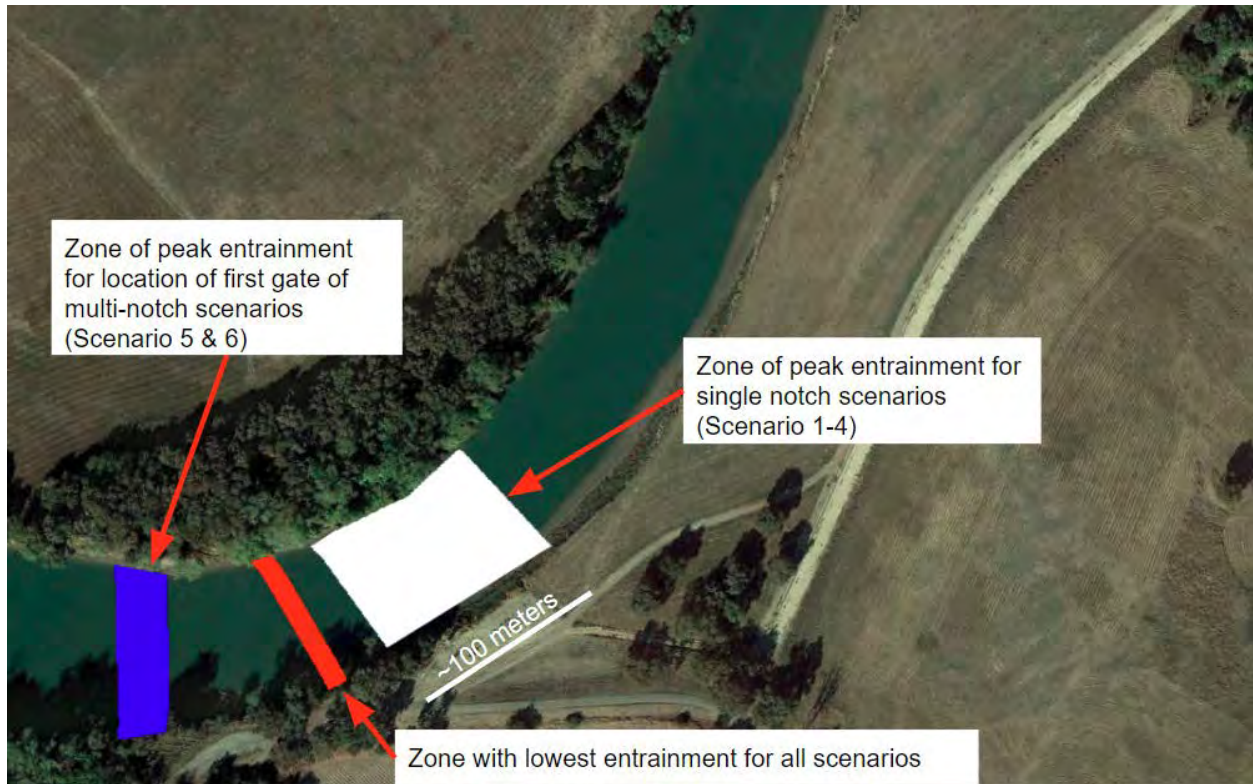
Figure 17 - Figure showing the location of maximum and minimum entrainment for fall run for all scenarios overlaid on an aerial photograph of the study area.
