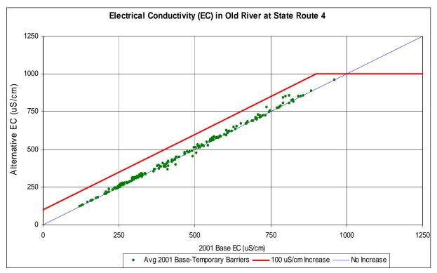
**Figure 3-3.** DSM2-Simulated EC (µS/cm) in Old River near SR 4 Bridge (CCWD Los Vaqueros Intake) for 1976–1991 with Temporary Barriers Compared with No-Barriers Conditions
