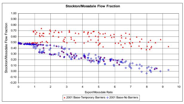
**Figure 3-2.** DSM2-Simulated Monthly San Joaquin River Flow at Stockton for 1976–1991 and the Stockton/Mossdale Flow Fraction as a Function of the Export/Mossdale Ratio for Temporary Barriers and No-Barriers Conditions (2001 Conditions)
