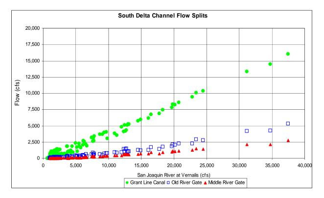
**Figure 3-6.** DSM2-Simulated Flow Distribution in Old River, Middle River, and Grant Line Canal as a Function of San Joaquin River Flows at Vernalis
