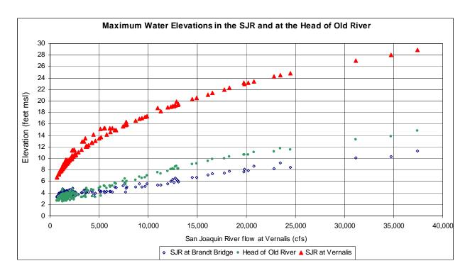
**Figure 3-4.** DSM2-Simulated Maximum Water Levels in the San Joaquin River at the Head of Old River and at Brandt Bridge, as a Function of the San Joaquin River Flow at Vernalis
