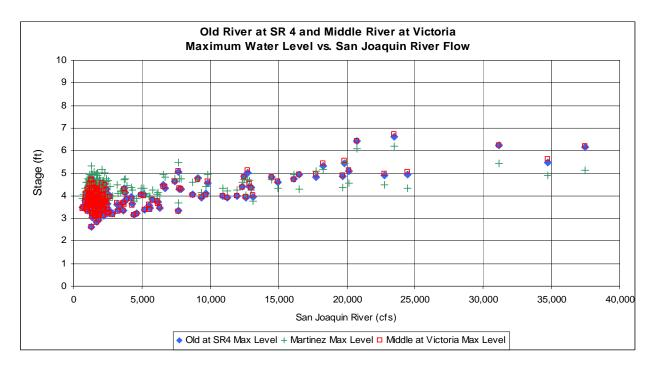
**Figure 3-7.** DSM2-Simulated Maximum (High Tide) Water Elevation (feet msl) in Old River and Middle River as a Function of San Joaquin River Flow at Vernalis (cfs) and High Tide Elevation at Martinez (Suisun Bay)
