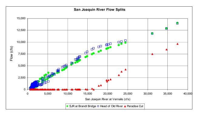
**Figure 3-5.** DSM2-Simulated San Joaquin River Flow Diversions at Paradise Cut and the Head of Old River as a Function of San Joaquin River Flows at Vernalis
