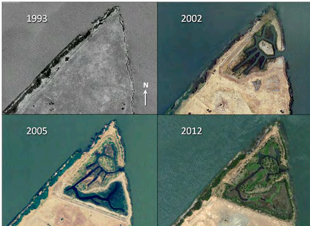
Figure 10. Mosaic of Decker Island State Wildlife Area development at north end of island. Channels dug have eventually filled with sediment and non-native aquatic plants (light green areas are predominantly water hyacinth). (DWR figure)
