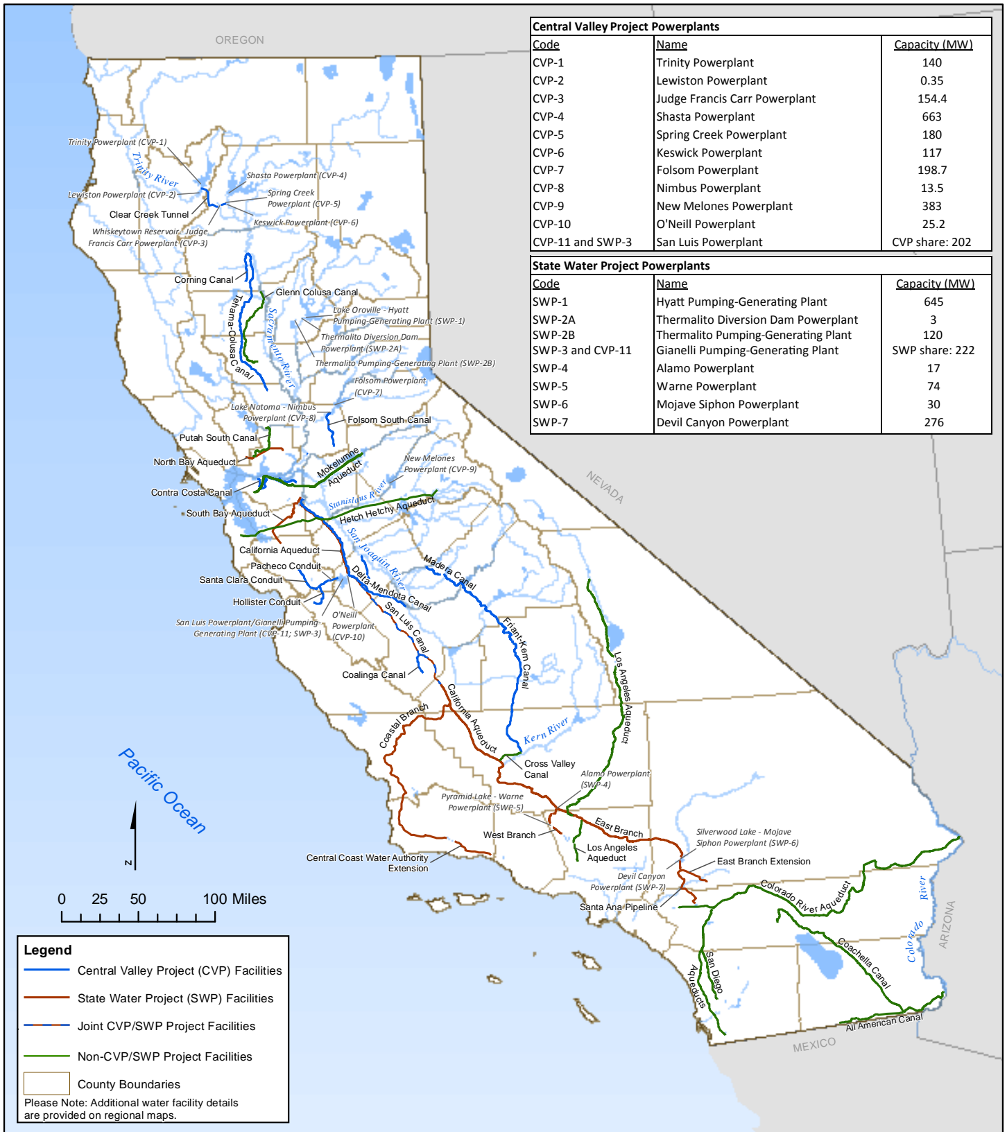
Figure 8.1 Central Valley Project and State Water Project Hydroelectric Generation Facilities
