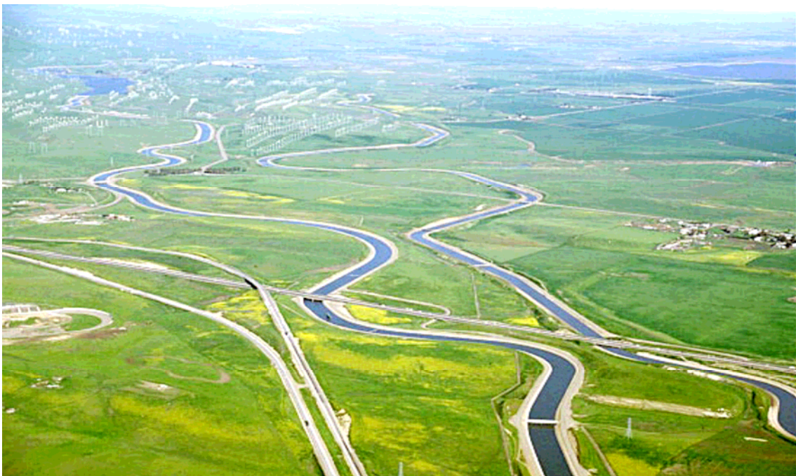
Photograph 5.1-18. SWP California Aqueduct (on Left) and CVP Delta-Mendota Canal (on Right) Conveying Water from the Delta (Top of Photograph) South to O'Neil Forebay and San Luis Reservoir (Source: California Department of Water Resources.)
