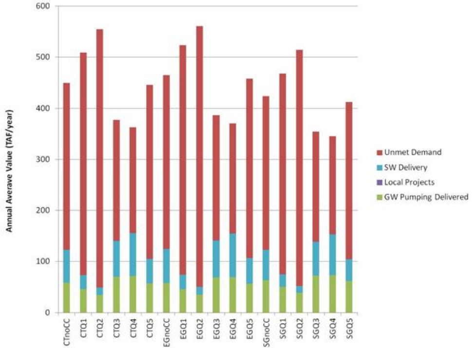
Figure 3-87. Average Annual Supplies and Unmet Demand in the Eastside Division in each Scenario
