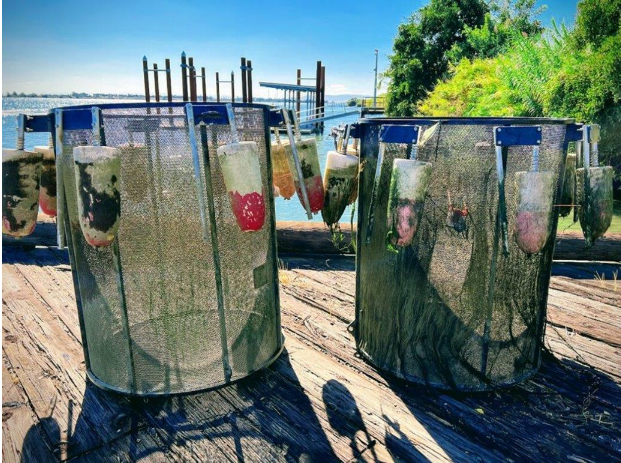
FIGURE 22. CAGES REMOVED FROM THE WATER AFTER THE SIX WEEK DEPLOYMENT. THE CAGE ON THE LEFT WAS EXCHANGED EVERY TWO WEEKS, WHEREAS THE CAGE ON THE RIGHT WAS SCRUBBED ONCE PER WEEK. THE BIOFOULING COMMUNITY IS APPARENTLY MUCH LIGHTER ON THE CAGE THAT WAS EXCHANGED.
