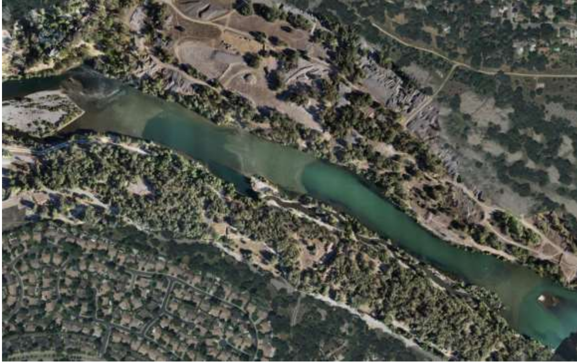
Figure 8. Aerial view of completed project at Lower Sailor Bar, September 30, 2022. The two side channels can be seen on the south side of the river and the three lighter colored areas are the gravel placements.
