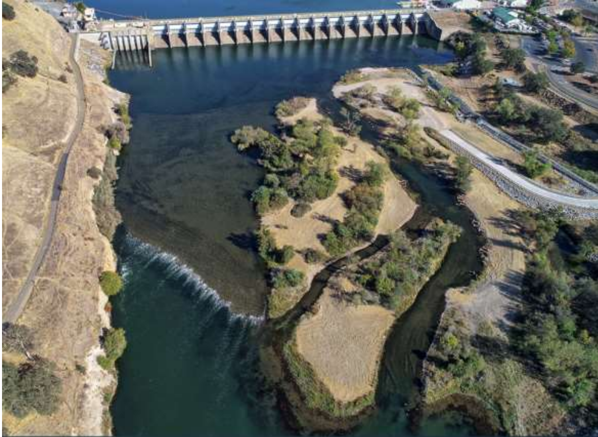
Figure 9. Completed project at Nimbus Basin, October 22, 2022. Salmon can be seen holding along the upstream part of the riffle (small black dots).
