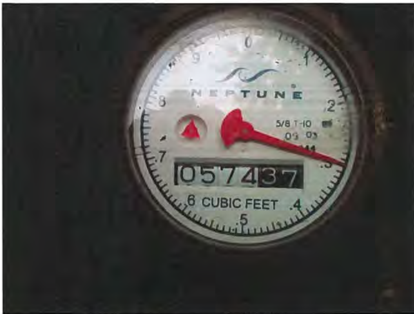
Figure 4: A typical older water meter reading in cubic feet (CF) reading = 54,437 CF or 574 BU
