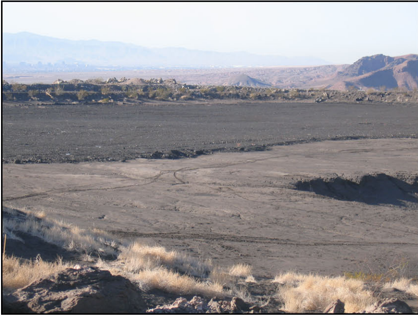
Photo 25 – Tailings pond 1 facing NW. Left side of tailings with waste manganese nodules; right side without. January 9, 2007.
