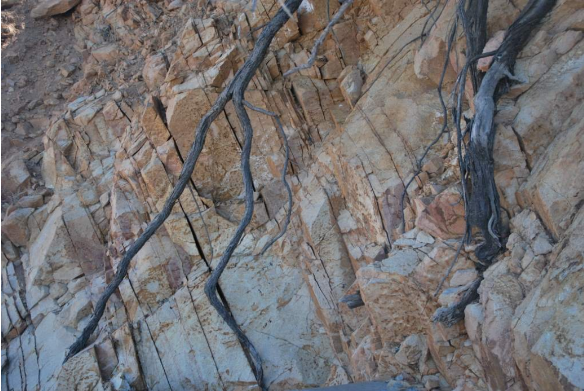
Photograph 2. Closely Spaced Fractures in the Fine-Grained Granite at the Bartlett Dam
