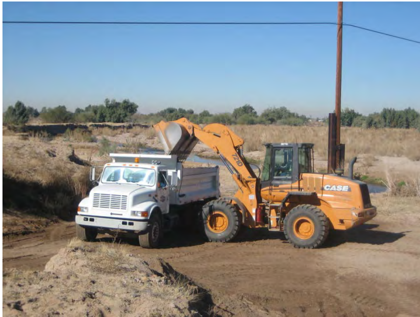
Photo Number: 00401072011 Photo Taken by: Carol Jean Hansen Narrative: The Case front end loader loading the Metro Water District dump truck.
