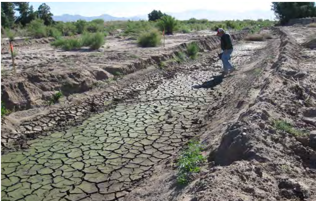
Photo 12. – Mudcracks in Channel 1 after 7 Days of Drying during First Maintenance Event. Brad Despain is crossing channel.
