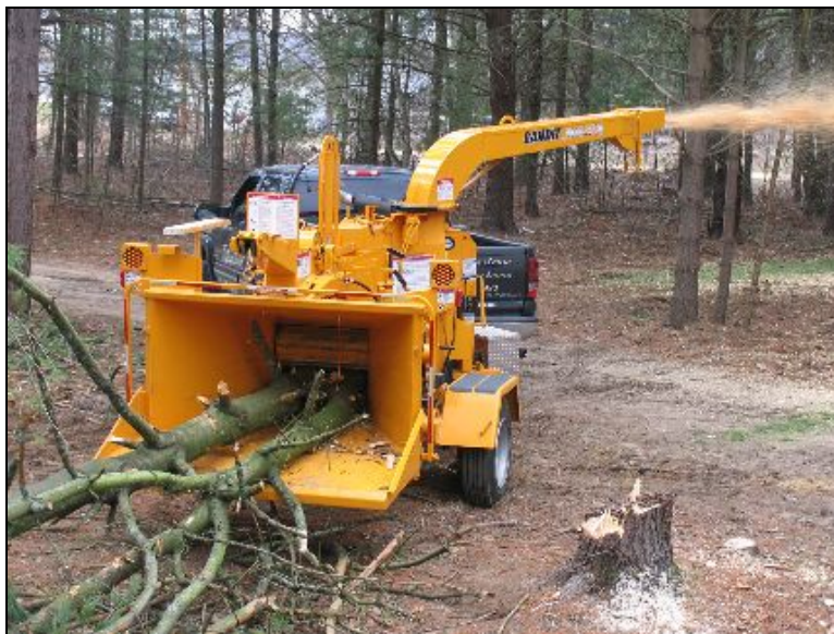
Figure 7. 15 inch diameter, hand fed chipper.
