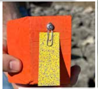
Water sensitive paper strip after a test flight showing droplet pattern.
