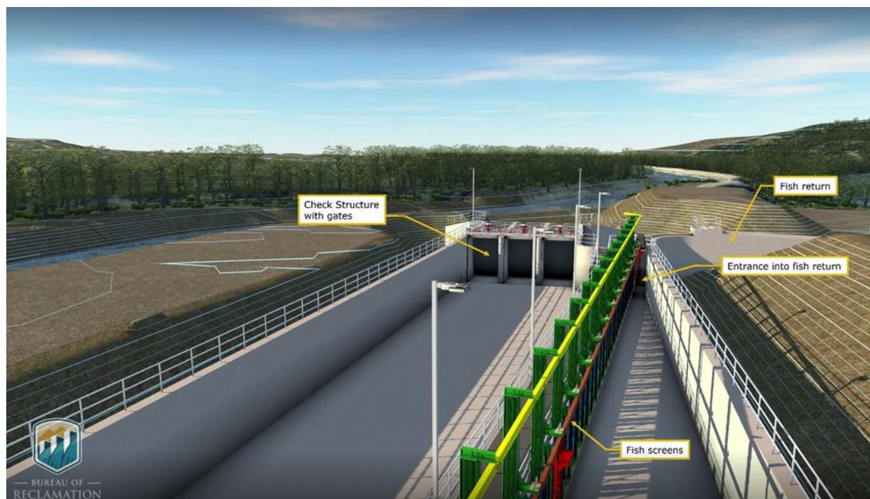
Figure 6: Fish Screen, Fish Return, and Check Structure
