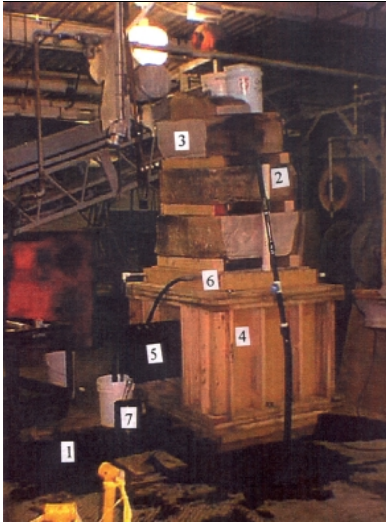
Figure 3 – Pipe box test apparatus includes a pump in the floor sump (1), standpipes (2), ballast (3), pipe box (4), drain pipe (5), overflows (6), and outflow sieves (7).
