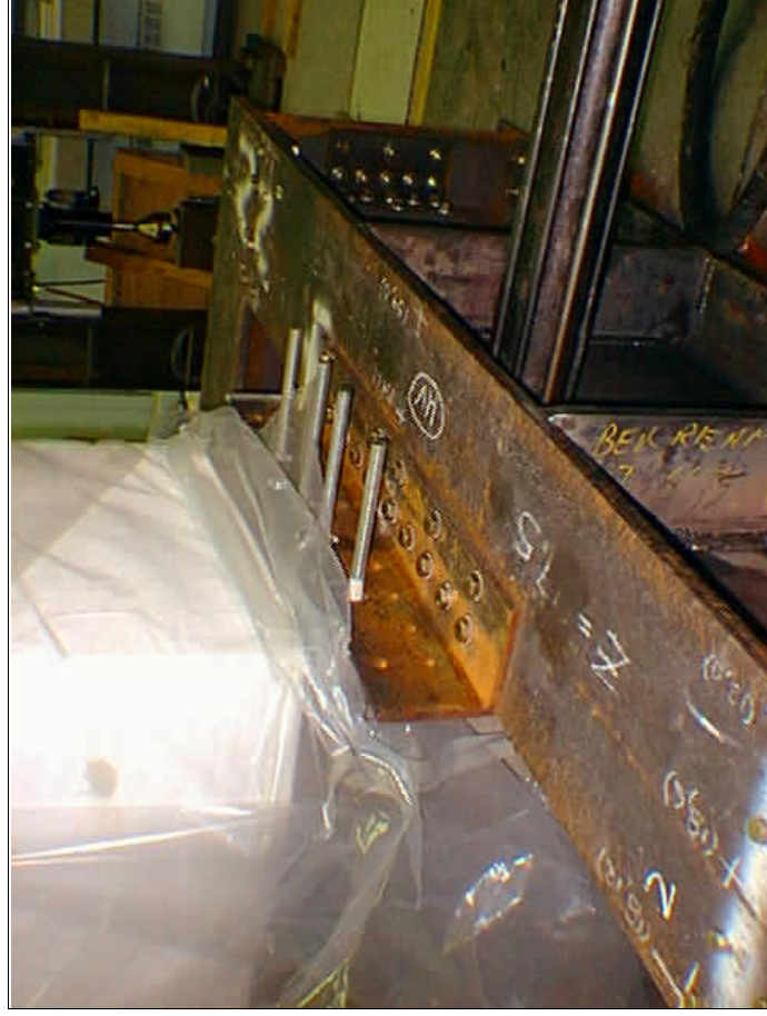
A view of one of the brackets that helps hold the model in the table.
