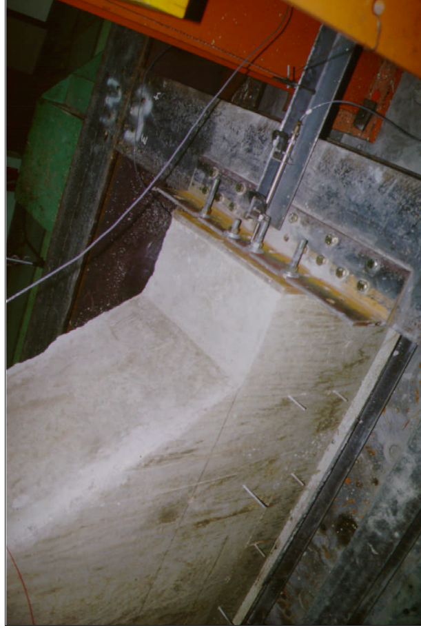
A view of the bracket and LVDT near the back of the model.
