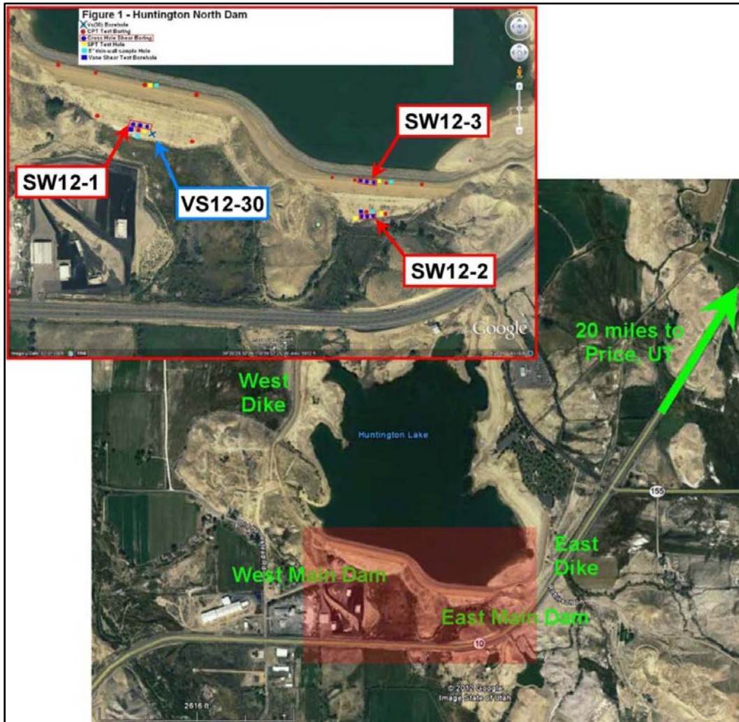
Figure 40 – Locations of various 1D crosshole seismic profiling surveys (red labels) and 1D FWS surveys (blue labels) conducted at both the west and east main sections of the Huntington North Dam facility in Utah.
