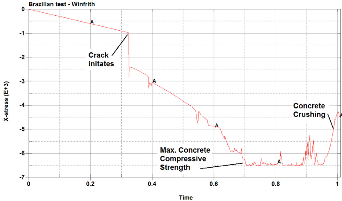
Figure 5.9. — Change of vertical stress at the specimen center with the load increments.
