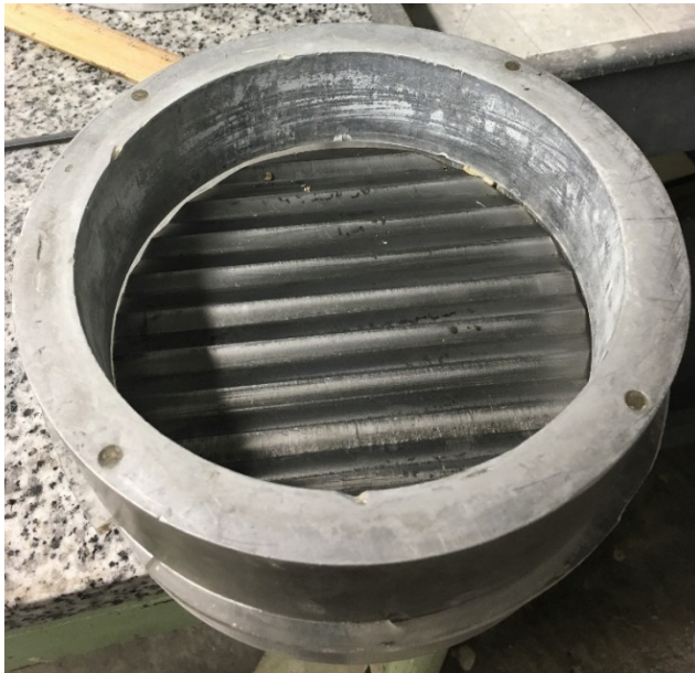
Figure 7 - Sawtoothed aluminum specimen ready for hydrostone pour. Note 0.2 in plexi-glass spacer between upper and lower rings.
