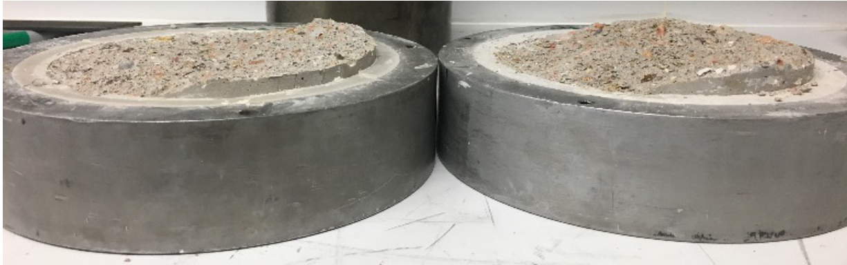
Figure 15 - Specimen CC-3 after CNL testing (break bond at 40 psi). Inclined breaks are typical with this type of test, with the sliding occurring in the “down-hill” direction. Specimen top on the left side of photo.
