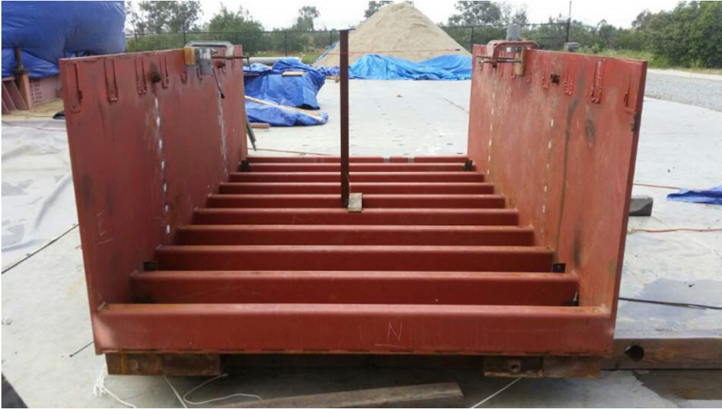
Figure 2. Photograph of the model spillway structure (9.3 ft. in length out of plane).
