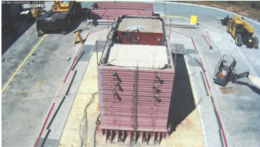
Figure 1. Photograph of the 15.2 ft. high, 22 ft. long, and 9.6 ft. wide laminar soil container on the shake table.
