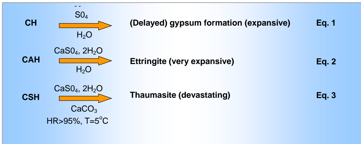
Figure 8: The mechanisms of delayed gypsum, ettringite and thaumasite formation
