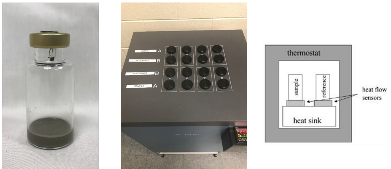
Figure 3. Paste sample (approx. 5 grams) used for isothermal calorimetry.
