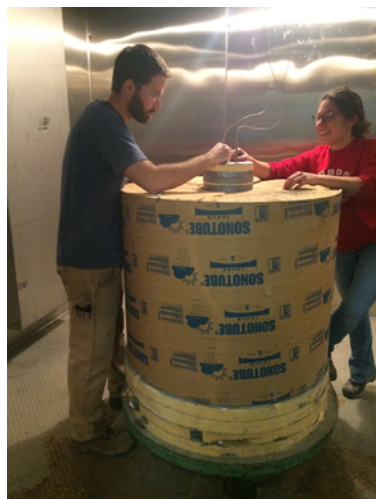
Figure 2. Test specimen for adiabatic temperature rise and room configuration.
