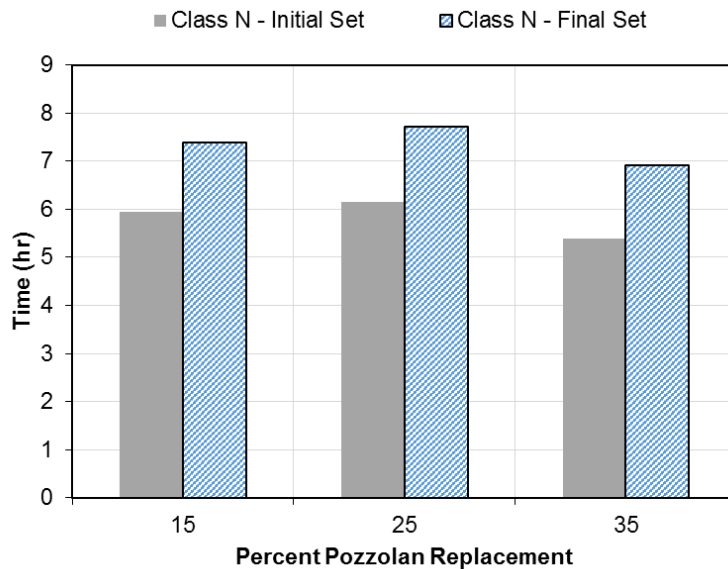
Figure 1. Initial and final setting time via penetrometer (ASTM C403).
