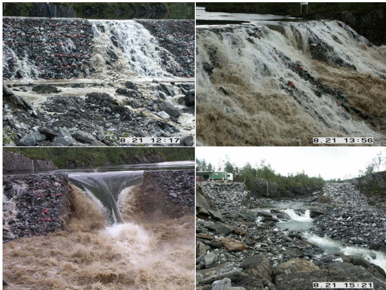
Figure 23.—Photos from the test of Norway embankment 1-03.
