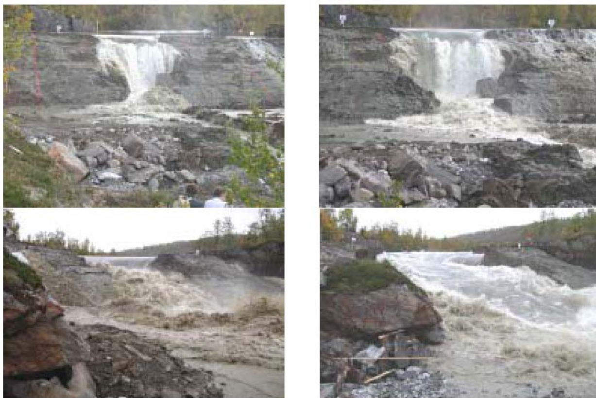
Figure 16.—Breaching of the Norway 1 clay embankment. Note that there is minimal drop in the water surface upstream from the test dam, even after breach is fully complete. The
